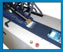
Fast, Easy and Flexible: The Product Attaching System's card feeder is synchronized for a superior tolerance range—you can place two cards on one piece.
